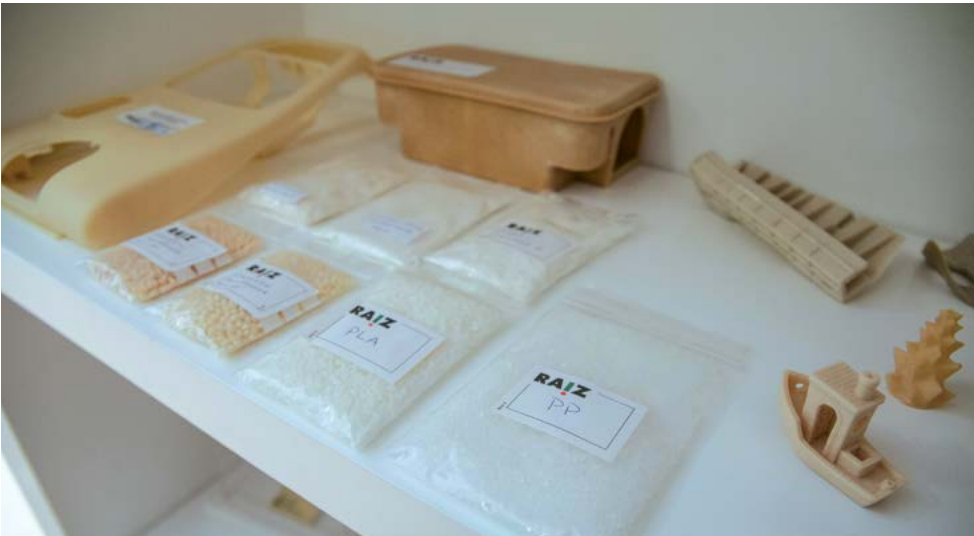
Biocomposites: cellulose fibres are mixed with thermoplastic materials, preferentially bioplastics.
