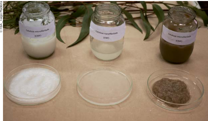
Micro- and nanofibrillated celluloses are an example of the forest-based bioeconomy and have been tested in paper production, to improve mechanical strength properties.
